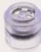
MODEL #157 - MANUAL RELIEF BLEED VALVE 5/8" PICTURED IN POLYCARBONATE WITH KALREZ® O-RING O.D. at 5/8" (15.88mm) Length at 0.630" (16.00mm) Plastics: Polypropylene, Nylon, Acrylic, Acetal, PVDF, Polycarbonate, Ultem®, ABS O-rings: Buna-N, EPDM, Viton®, Silicone, Fluorosilicone, Aflas®†, Kalrez®† Springs: 0.11 - 8 PSI
