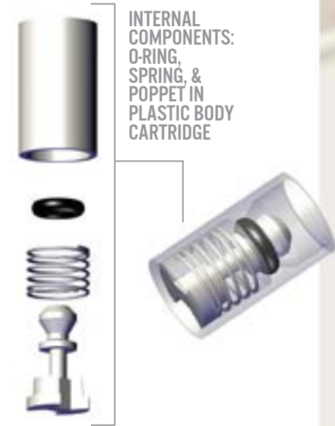
MODEL #170 - STANDARD CARTRIDGE 3/4" PICTURED IN GREEN POLYPROPYLENE & IN ACRYLIC WITH SILICONE O-RING O.D. at 3/4" (19.05mm) Length at 1.125" (28.58mm) Plastics: Polypropylene, Nylon, Acrylic, Acetal, PVDF, ABS O-rings: Buna-N, EPDM, Viton®, Silicone Springs: 0.16 - 3 PSI
