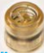
MODEL #150 - STANDARD CARTRIDGE 5/8" PICTURED IN RADEL® WITH AFLAS® O-RING O.D. at 5/8" (15.88mm) Length at 0.630" (16.00mm) Plastics: Polypropylene, Nylon, Acrylic, Acetal, PVDF, Polycarbonate, Ultem®, ABS, Radel® O-rings: Buna-N, EPDM, Viton®, Silicone, Fluorosilicone, Aflas®†, Kalrez®† Springs: 0.11 - 8 PSI
