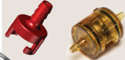
MODEL #302 - BARBED 1/8" PAIRED WITH SAME MODEL #302 PICTURED IN ULTEM® WITH BUNA-N O-RINGS Tubing I.D. at 1/8" (3.18mm) Plastics: Polypropylene, Nylon, PVDF, Ultem®, ABS O-rings: Buna-N, EPDM, Viton®, Silicone, Fluorosilicone, Aflas®†, Kalrez®† Springs: 0.11 - 20 PSI
