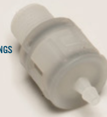
MODEL #330 - MANUAL RELIEF PAIRED WITH MODEL #302 PICTURED IN RED POLYPROPYLENE Unique style provides pressure or vacuum relief at the touch of a button. Threaded for panel mounting; 5/8-18 thread pitch Plastics: Polypropylene O-rings: Buna-N, EPDM, Viton®, Silicone, Fluorosilicone, Aflas®†, Kalrez®†
