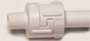
MODEL #361 - SMOOTH STEM 3/8" PAIRED WITH MODEL #314 PICTURED IN ABS Tubing I.D. at 3/8" (9.525mm) Plastics: Polypropylene, Nylon, PVDF, Ultem®, ABS, Radel® O-rings: Buna-N, EPDM, Viton®, Silicone, Fluorosilicone, Aflas®†, Kalrez®† Springs: 0.11 - 20 PSI
