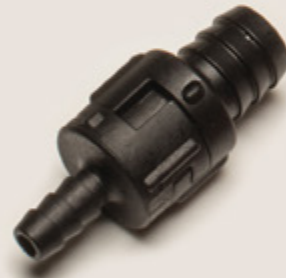
MODEL #308 - BARBED 1/2" PAIRED WITH MODEL #304 PICTURED IN BLACK NYLON Tubing I.D. at 1/2" (12.70mm) Plastics: Polypropylene, Nylon, PVDF, Ultem®, ABS O-rings: Buna-N, EPDM, Viton®, Silicone, Fluorosilicone, Aflas®†, Kalrez®† Springs: 0.11 - 20 PSI
