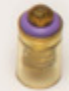
MODEL #110 - STANDARD CARTRIDGE 1/4" PICTURED ABOVE IN ULTEM® WITH EPDM O-RING & BELOW IN ACETAL WITH BUNA-N O-RING O.D. at 1/4" (6.35mm) Length at 0.500" (12.70mm) Plastics: Polypropylene, Nylon, Acrylic, Acetal, PVDF, Polycarbonate, Ultem®, ABS O-rings: Buna-N, EPDM, Viton®, Silicone, Fluorosilicone Springs: 0.09 - 20 PSI
