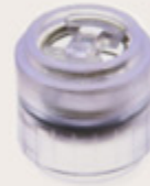
MODEL #157 - MANUAL RELIEF BLEED VALVE 5/8" PICTURED IN POLYCARBONATE WITH KALREZ® O-RING O.D. at 5/8" (15.88mm) Length at 0.630" (16.00mm) Plastics: Polypropylene, Nylon, Acrylic, Acetal, PVDF, Polycarbonate, Ultem®, ABS O-rings: Buna-N, EPDM, Viton®, Silicone, Fluorosilicone, Aflas®†, Kalrez®† Springs: 0.11 - 8 PSI
